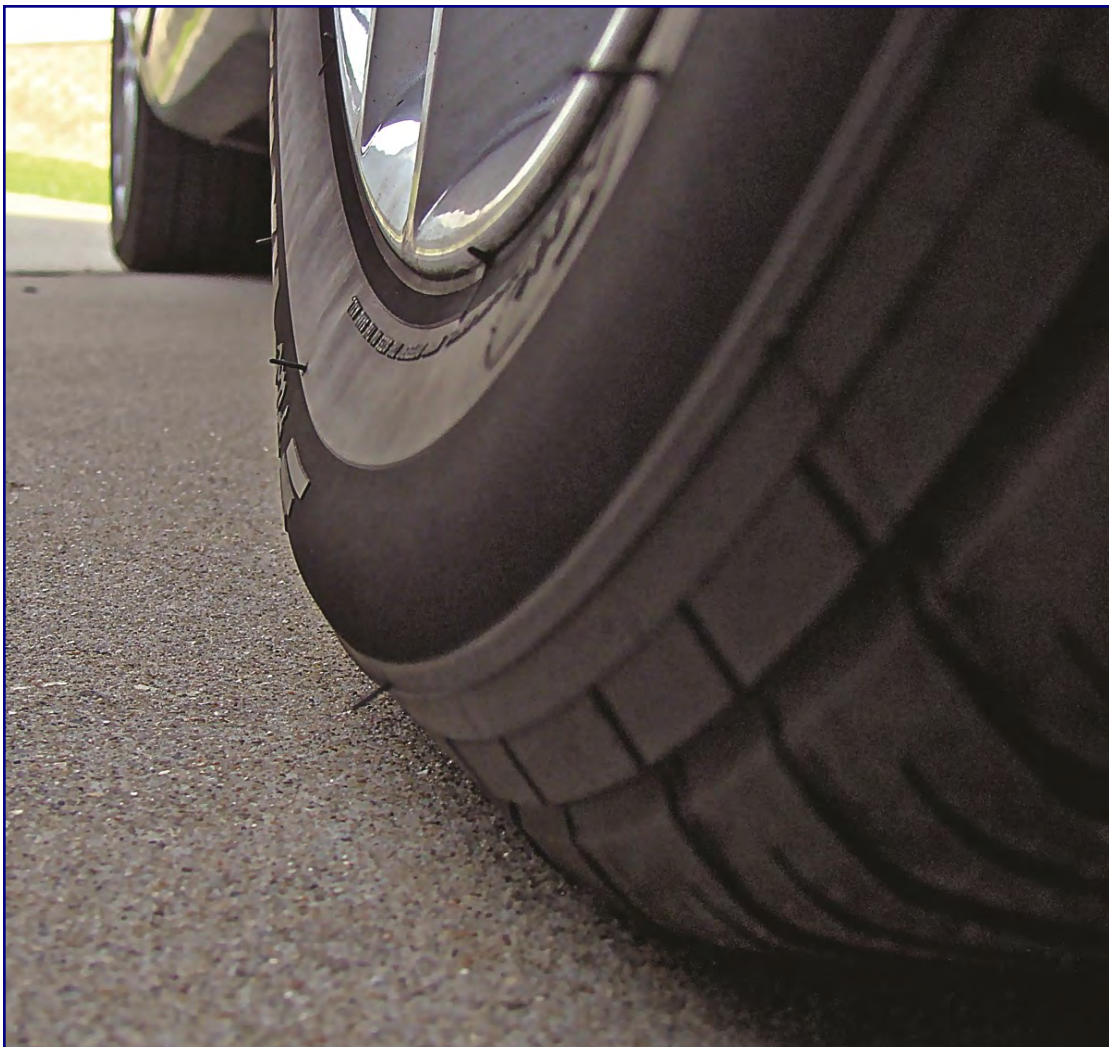
This low-profile car tire begins to bulge when tire pressure drops below 25 psi.
